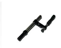
Very sturdy and solid holdfast, body with a  $\emptyset$  25 mm or 30 mm, for any board of your work-bench. Steel body, screw consists of a high quality trapezoidal thread. Holdfast dimensions are 25 x 360 mm or 30 x 360, the jaw length is 150 mm
